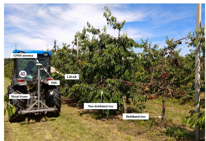
Fig. 1. The LiDAR sensor, GNSS rover antenna and IMU were installed on a metal frame and mounted on the tractor for scanning of non-defoliated and subsequently defoliated cherry trees at 80 DAFB.
